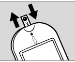
**2** Pull out the Check Strip, and *quickly* insert it back into the Meter (within 2 seconds).
